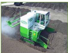
The **CMC SF 300** is the flagship for quality composting. Windrows with a width up to 3.4 m show very good properties for the production of high quality compost
