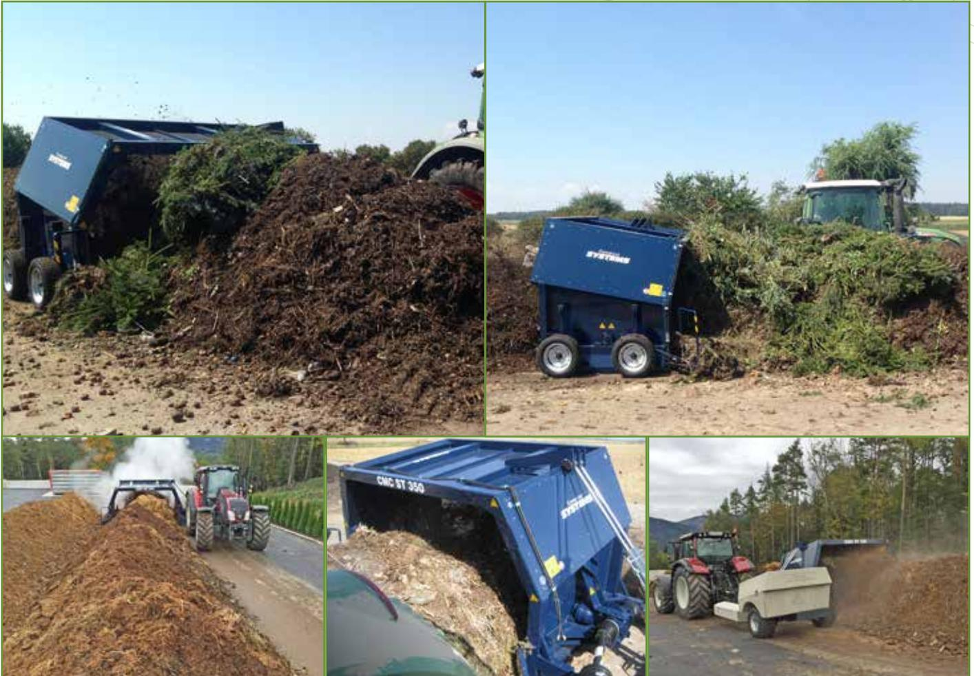
With a rotor length of 3.5 m and a heap cross-section of about 4 m<sup>2</sup>, Compost Systems expands its Agroline with the **CMC ST 350** for tractors above 100 hp. With or without a super creeper gear, the **CMC ST 350** works well with a push axle (option) even without creeper speed. The turner has a transport height of more than 4.6 m, which is not suitable
